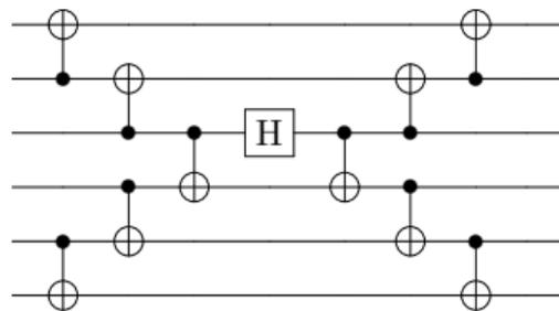
Figure: CNOT-based XOR measurement
