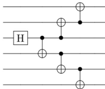
**Figure:** 6 qubit CNOT-based GHZ discriminator
