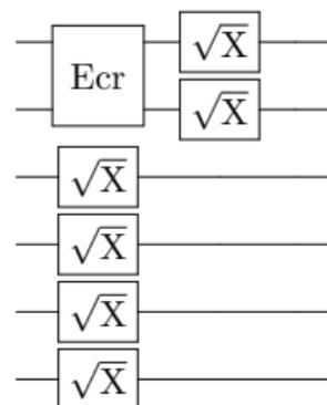
Figure: ECR-based short measurement
